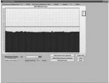
In this case for instance the power demand during normal operation could be reduced by 20% to 1433kW without harming process dynamics. The limit of 1433kW is set in the Eurotherm EPower master controller and Eurotherm patented load shedding feature takes care that the limit is never exceeded.
